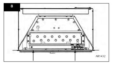
2.14 • Remove the 11 screws in the burner tray securing the burner assembly to the appliance. The burner assembly can now be removed by lifting it up and out of the appliance, Diagram 9.
